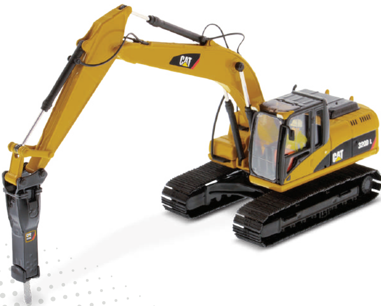
Excavator with Breaker
